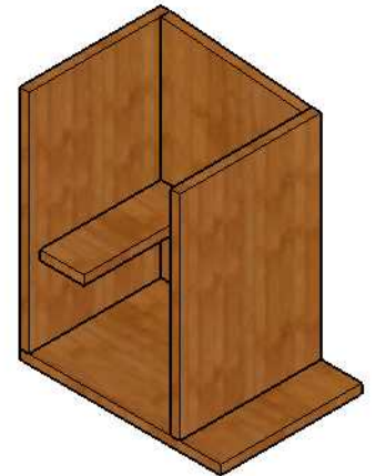
Attach Platform to Tall Side About 6in from Base. Front not shown.
